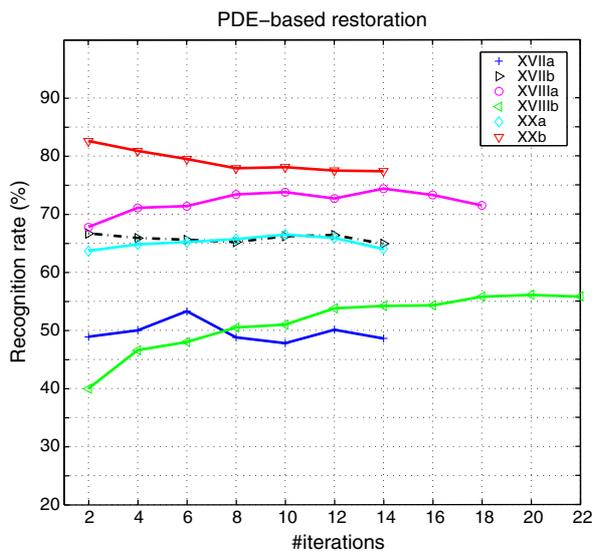
Fig. 16. Recognition accuracy as a function of the number of iterations when preprocessing images with the Perona–Malik PDE-based approach.
