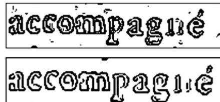
Fig. 3. Edges from a highly degraded word from set XVIII-b. From top to bottom: without regularization, after regularization by TV.
