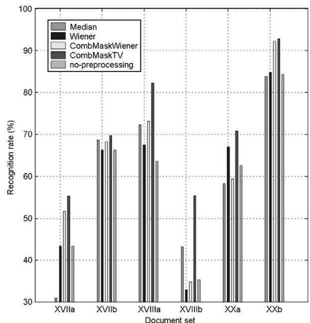
Fig. 15. Comparison of enhancement methods through character recognition accuracy (in%). Dictionary corrections are turned off.
