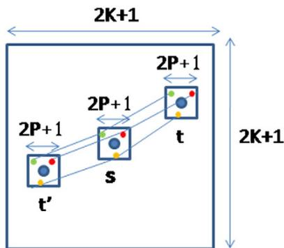
Fig. 5. NLmeans approach: two patches  $\Delta$  of size  $2P+1$  around  $t$  and  $t'$  within the size  $2K+1$  search window centered on  $s$ . The similarity measure between patches is computed from all pairs of points at the same location within patches.
