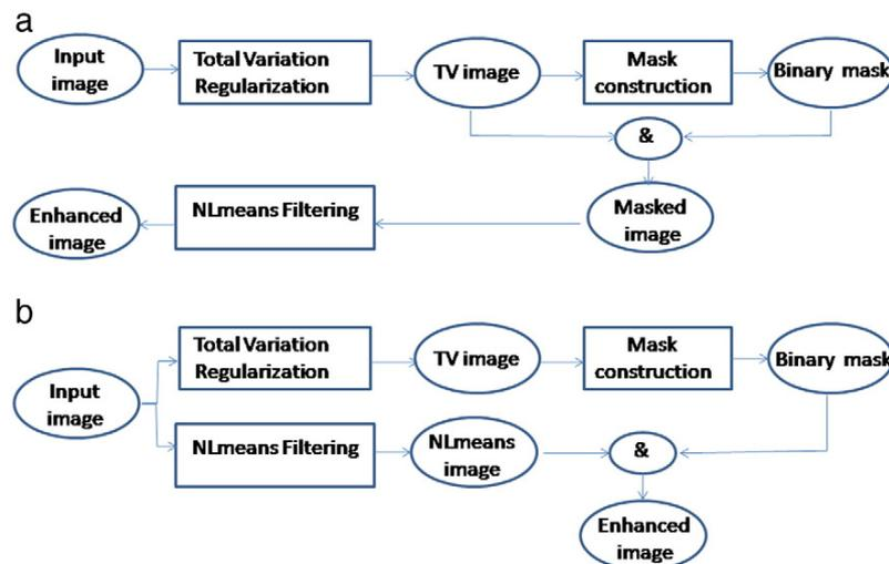
Fig. 1. Flowcharts of the two proposed enhancement methods combining TV regularization and NLmeans filtering. a) type-A combination b) type-B combination.
