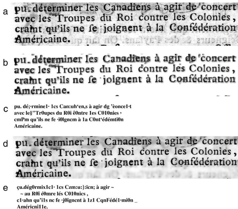
Fig. 17. a) Input image from set XVIIIa. b) type-A combination c) OCR result for the type-A combined image (dictionary corrections turned off) d) PDE processed image with six iterations and e) OCR result for the PDE-enhanced image.
