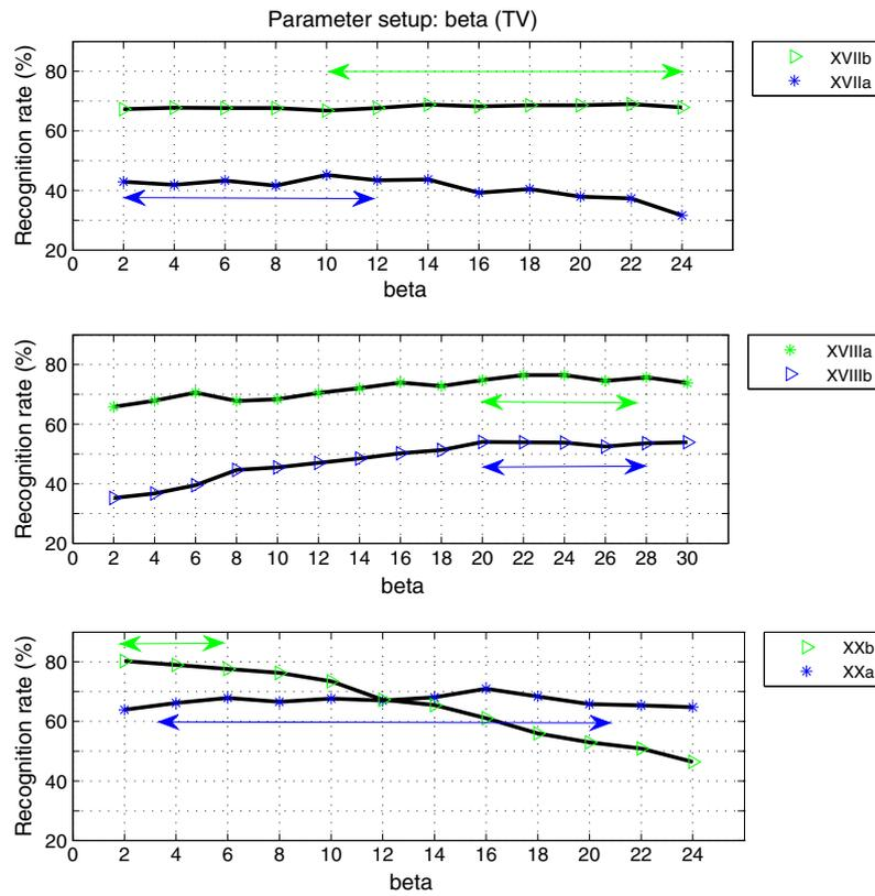
Fig. 10. Performance of TV regularization as a function of the  $\beta$  parameter. Arrows indicate for each set the range of operating values for  $\beta$ .
