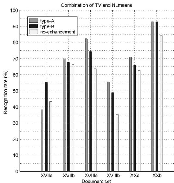
Fig. 14. Combination of TV and NLmeans. Performance of the combined methods (types A and B) through character recognition accuracy (in%).
