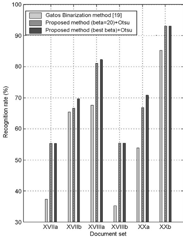
Fig. 18. Comparison of proposed enhancement method followed by Otsu binarization with the binarization method presented in [19]. Results for the proposed enhancement method are given for the default  $\beta=20$  and the best  $\beta$  values.
