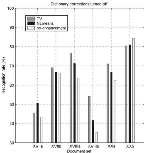
Fig. 11. Performance of TV regularization and NLmeans filtering as single enhancement methods (without combination). Dictionary corrections are turned off.
