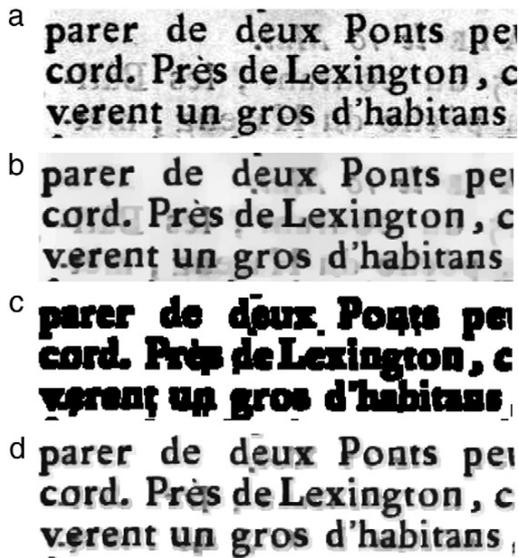
Fig. 4. a) Input image b) TV-regularized image c) mask and d) enhanced image resulting from the application of the mask on the TV image. Pixel values outside character regions are saturated to 255.
